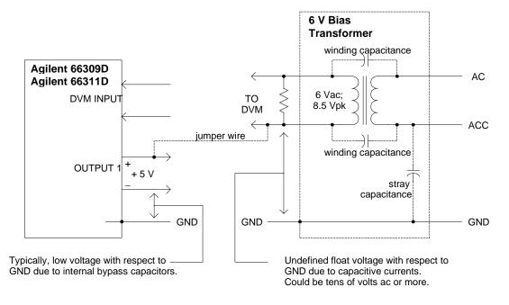
Figure 3-9. Measuring Circuits Floating with Respect to the Main Output
